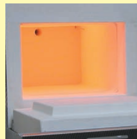
Muffle heated from four sides
