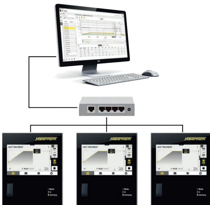
Example lay-out with 3 furnaces
