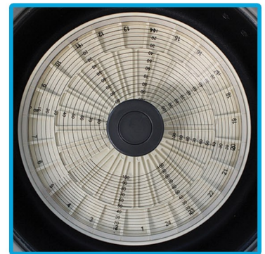
24-place capillary rotor with reading disc lid
