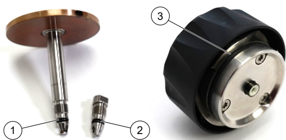
Fig. 32: O-rings on bearings and measuring cell lock
