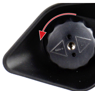
Fig. 24: Opening the measuring cell lock
