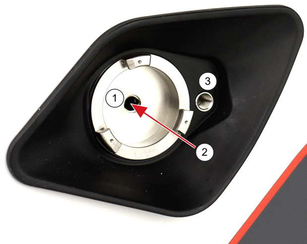
Fig. 29: How to clean the viscosity measuring measuring cell
