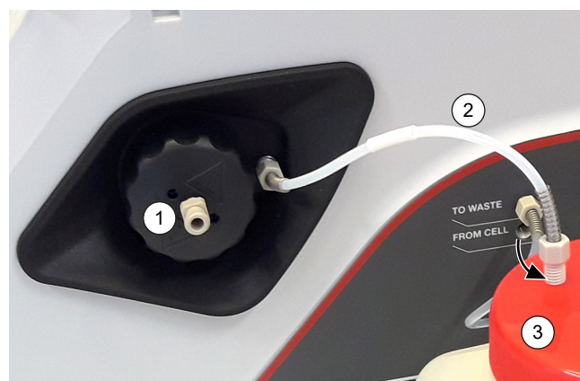
Fig. 15: Simple Fill - setup for syringe filling
