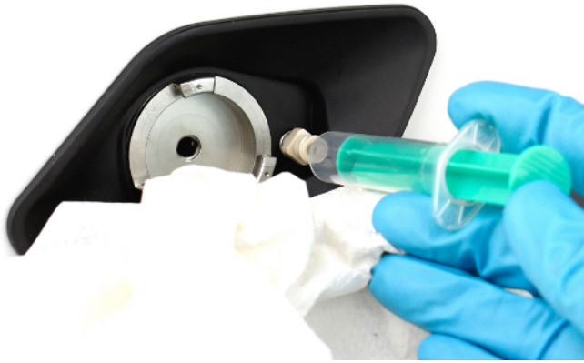
Fig. 30: Rinsing the measuring cell from the outlet
