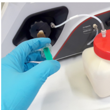
Fig. 18: Filling sideways with a 5 mL syringe
