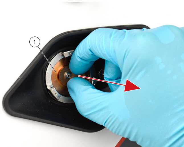
Fig. 26: Taking out the measuring rotor
