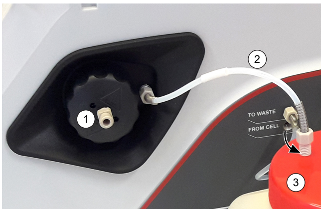
Fig. 18: Simple Fill - setup for syringe filling
