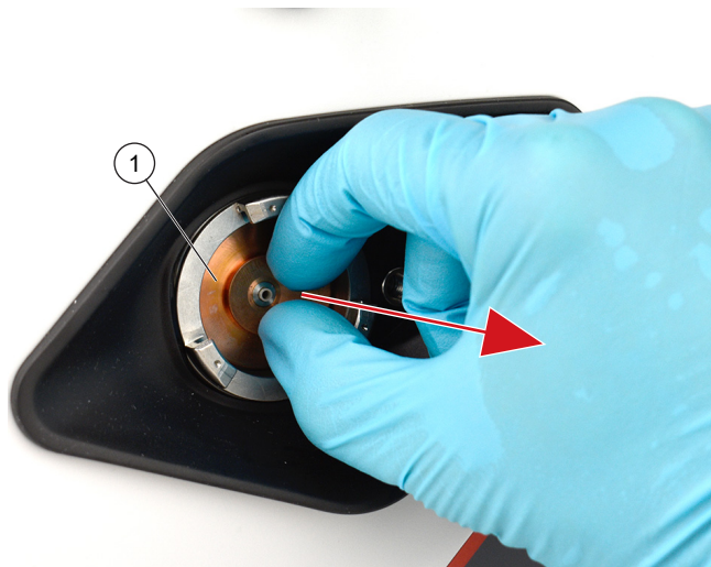
Fig. 31: Taking out the measuring rotor
