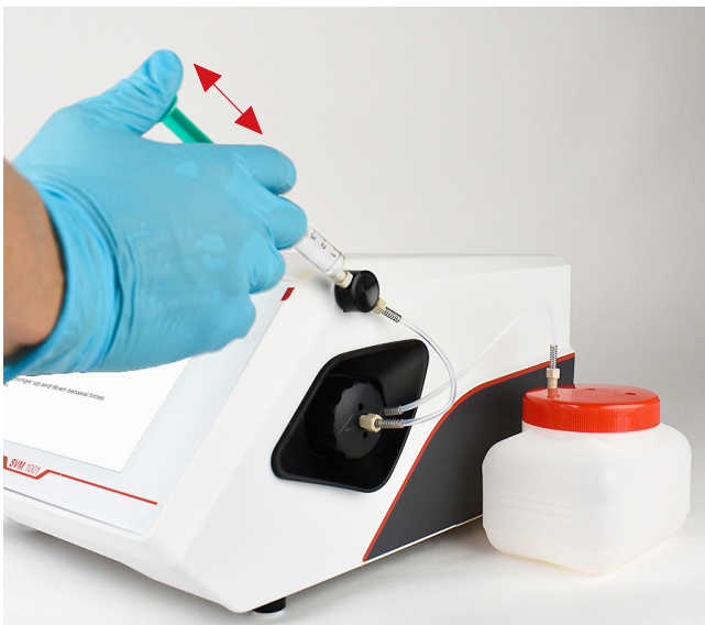
Fig. 24: Cleaning using a syringe – move the plunger
