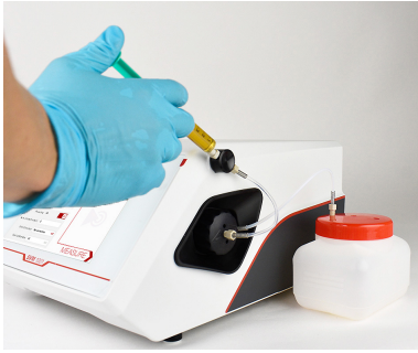
Fig. 21: Filling SVM 1001 with a 5 mL syringe
