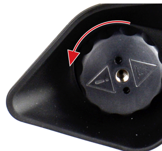
Fig. 29: Opening the measuring cell lock
