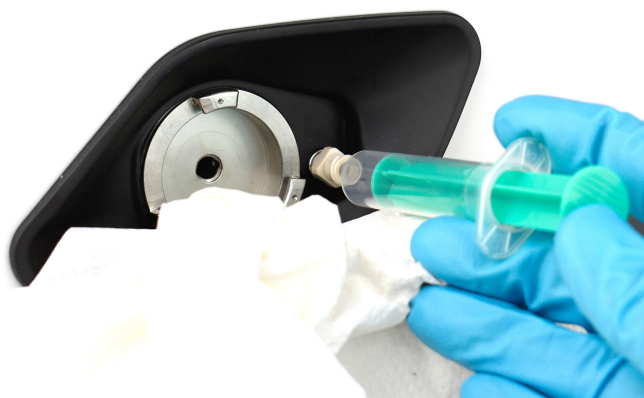
Fig. 35: Rinsing the measuring cell from the outlet
