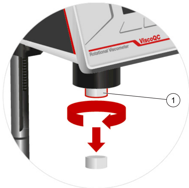
Fig. 4: Removing the transport protection
