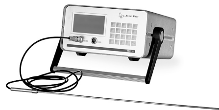
Fig. 4: MKT 50 with connected sensor
