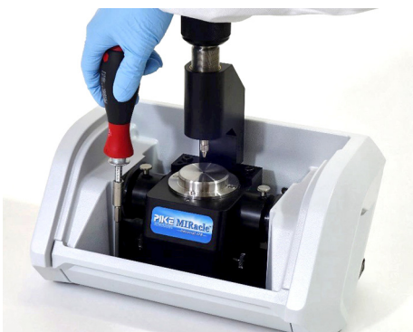
Figure 6: Fastening the captive screws with the Torx T25 screwdriver.
