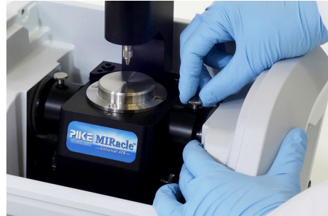
Figure 7: Loosen the knurled screws to adjust the purge tubes on both sides of the cell module, then tighten them again.
