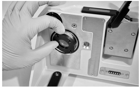
Fig. 8: Removing the KBr window
