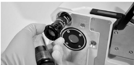
Fig. 11: Removing the drying cartridge
