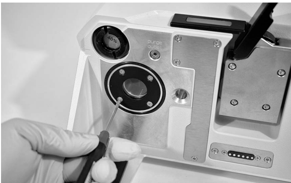
Fig. 7: Removing the fixing screws
