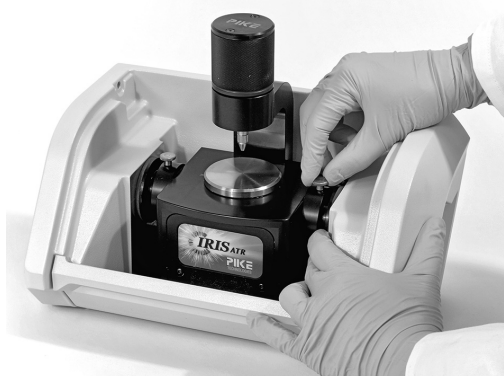
Fig. 6: Mounting a third-party cell and fixing the purge tubes
