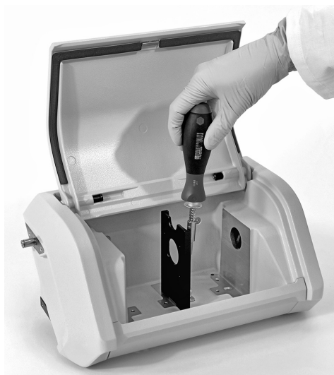
Fig. 5: Mounting the transmission cell holder
