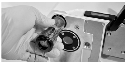
Fig. 10: Unscrewing the drying cartridge
