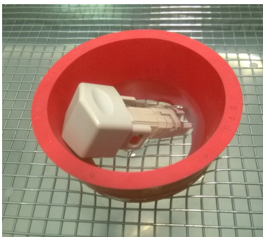
Fig. 48: The Univette was placed in an ethanol-filled quartz cuvette and ultrasonicated.
