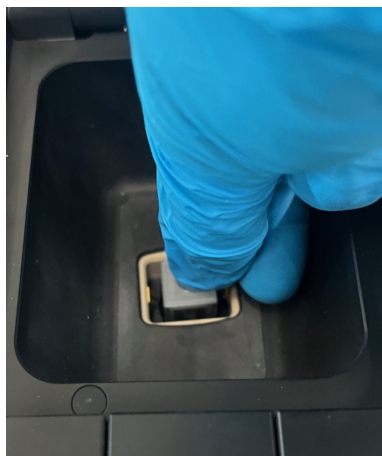
Fig. 21: Pressing the UVette® into place
