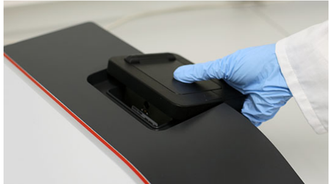
Fig. 50: Removing the cuvette module. This procedure is identical for the BM 11 cuvette module (depicted here) and the FM 11 cuvette module.
