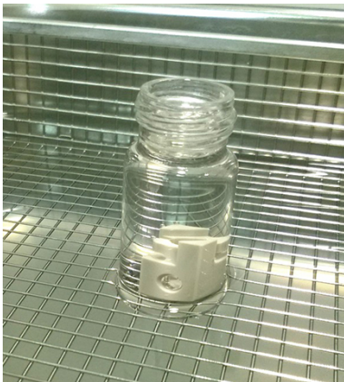
Fig. 49: Low-volume accessory undergoing ultrasonic treatment in an ethanol-filled glass bottle
