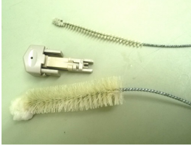
Fig. 47: The Univette electrodes can be cleaned with bottle cleaning brushes to remove protein and salt residues
