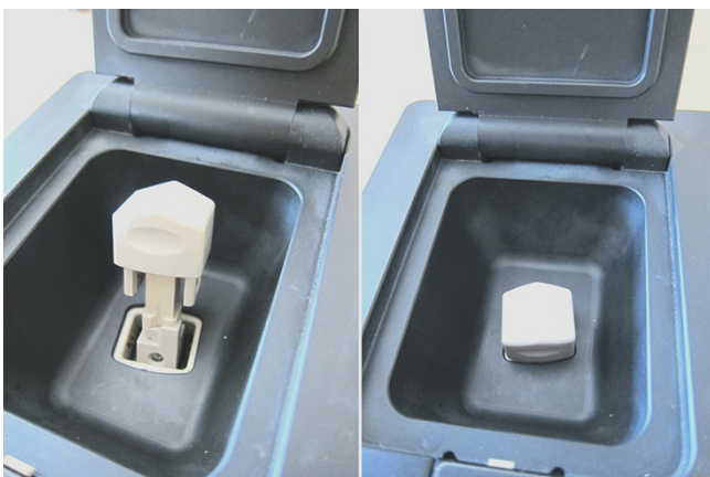
Fig. 33: Inserting the Univette and low-volume accessory After measurement, clean the Univette as described in Section 8.3 [▶ 27].
