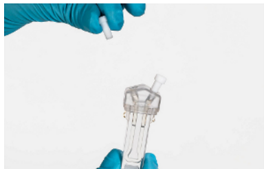
Fig. 23: Inserting the Luer plugs. Note that the figure refers to a discontinued version of the Omega cuvette, but that the procedure is identical for all types of Omega cuvettes.
