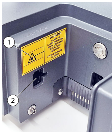
Fig. 1: Safety signs and laser aperture on the front surface of the module cavity
