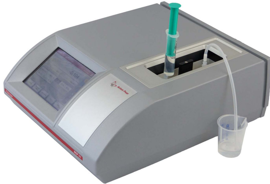
Fig. 7 - 3 Filling the cell with a syringe
