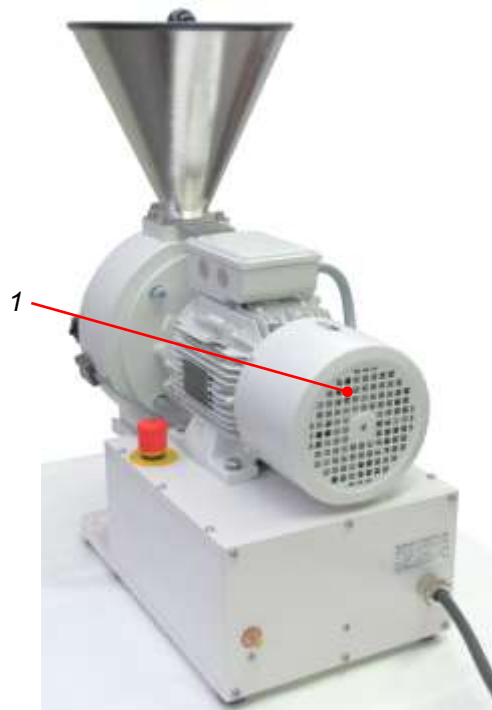
Fig. 12: Ventilation grille on the rear side
