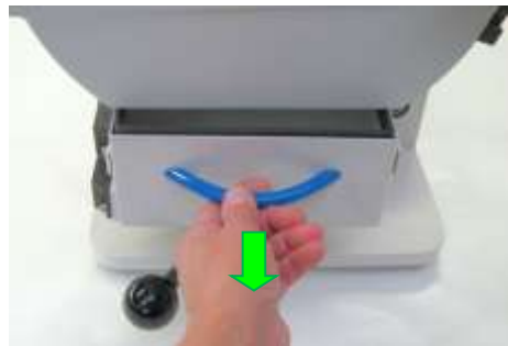
Fig. 25: Pulling out the collector
