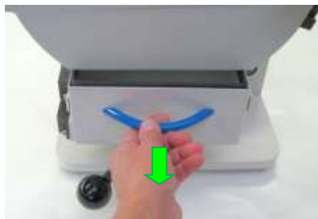
Fig. 23: Pulling out the collector
