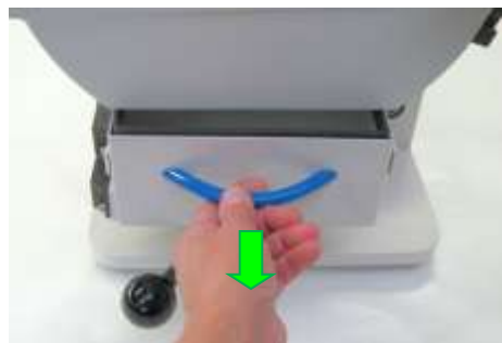
Fig. 14: Pulling out the collector
