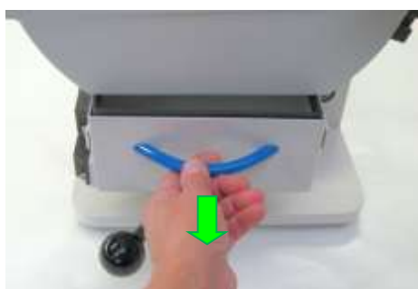
Fig. 21: Pulling out the collector
