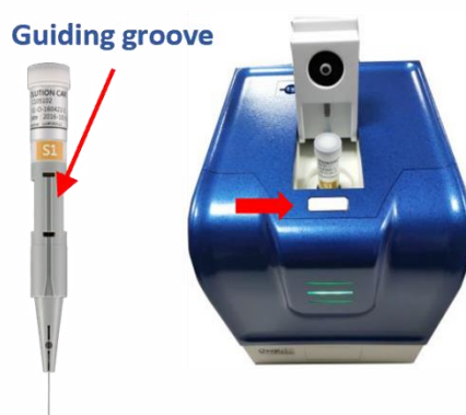
Figure 15 The guiding groove of the cartridge shall face the front
