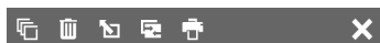
Fig. 16: Example of an action control for selecting and then removing, exporting, comparing, or printing the selected items
