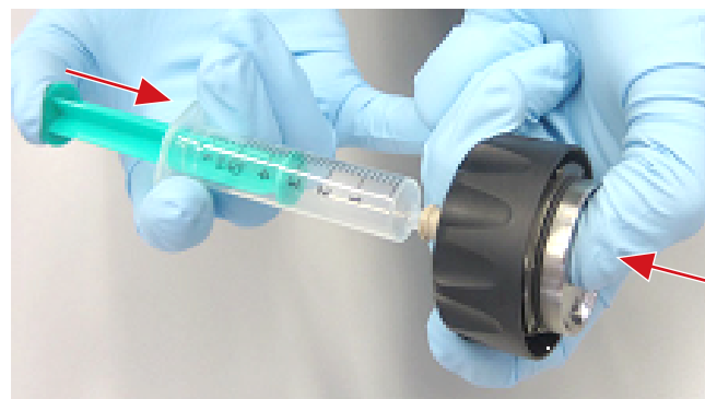
Fig. 22: Leak test measuring cell lock
