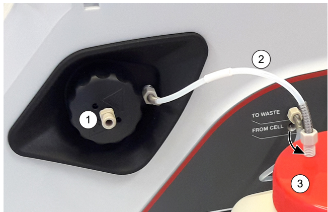
Fig. 15: Simple Fill - setup for syringe filling
