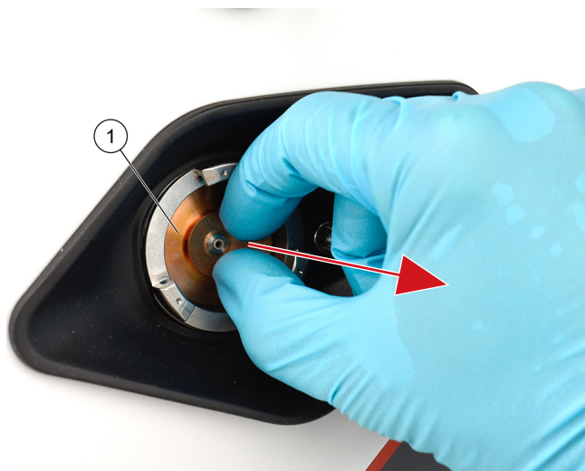
Fig. 26: Taking out the measuring rotor
