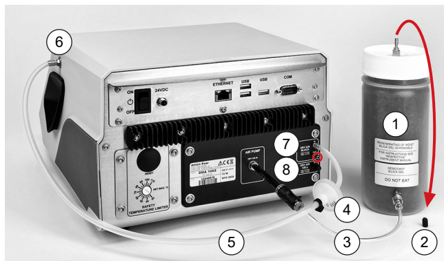
Fig. 8: Example: Removing condensation from the measuring cell block with the internal air pump
