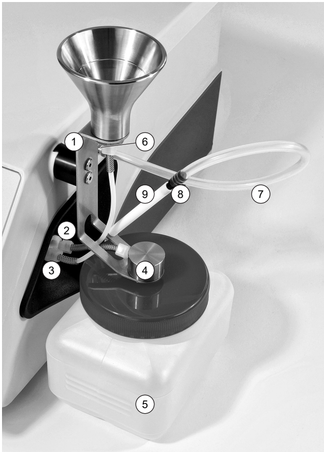
Fig. 5: Mounting the funnel, all hoses, and the waste vessel
