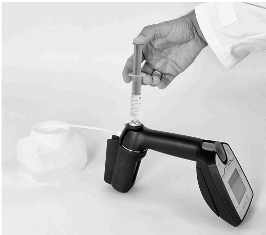
Fig. 10: Filling sample with a syringe
