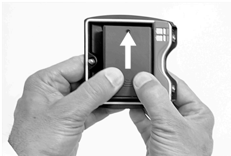
Fig. 14: Removing the cover of the battery compartment
