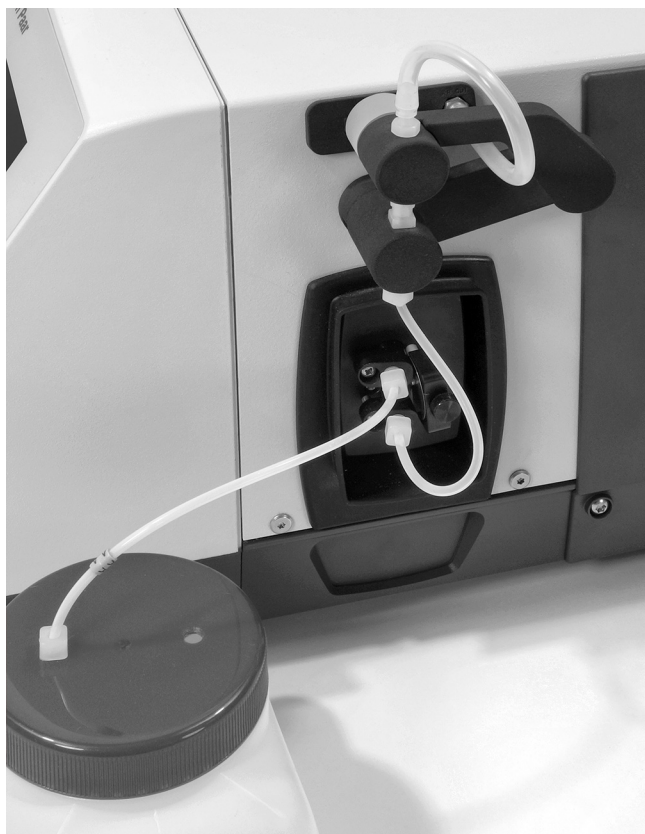
Fig. 12: Drying the measuring cells
