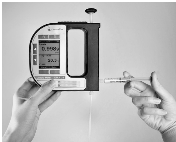
Fig. 8: Filling sample using the plastic syringe
