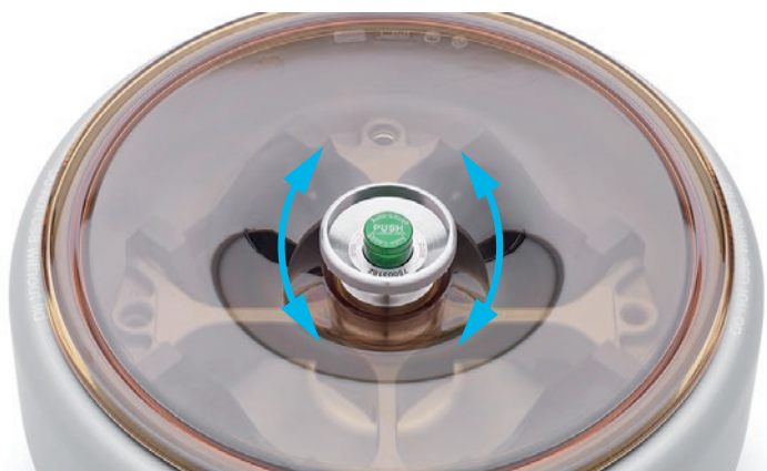
Figure 2-10: Turn the rotor knob
