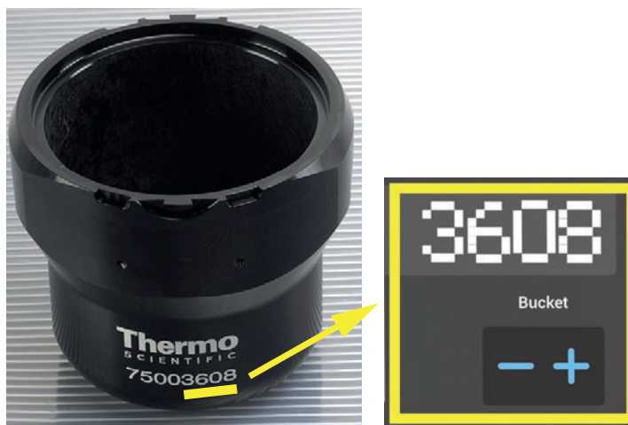
Figure 2-19: Setting the Correct Bucket Code
