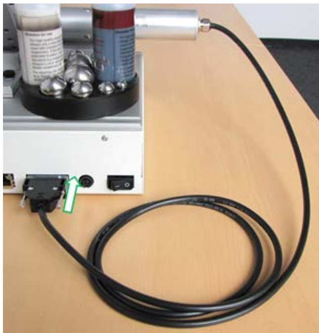
Fig. 14: Connecting motor to rear panel
