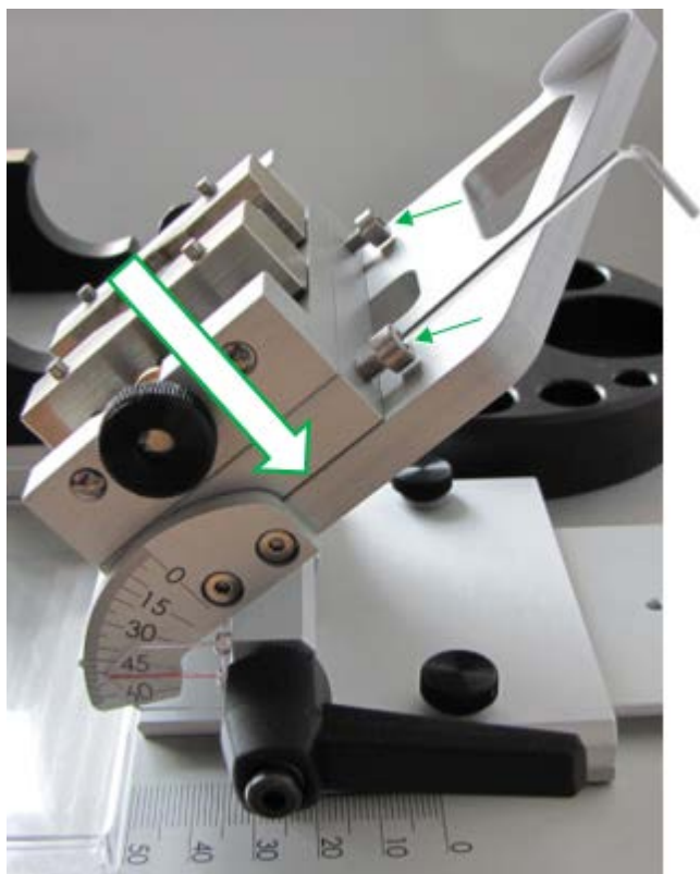
Fig. 21: Securing the sample holder (keeping it pressed against table) for mounting it on table
