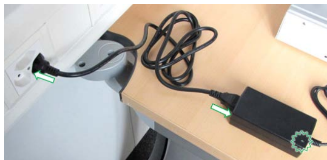
Fig. 17: Connecting main power cord to power supply and power outlet
