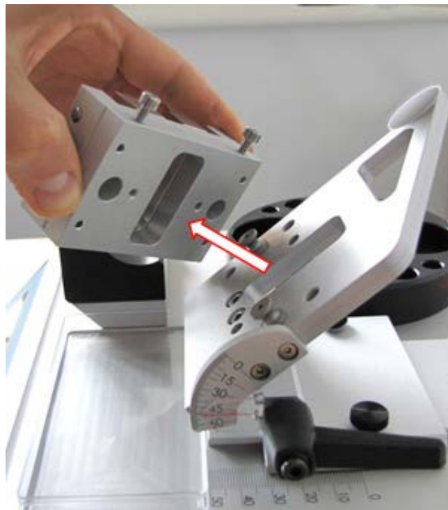
Fig. 24: Removing sample holder from table
