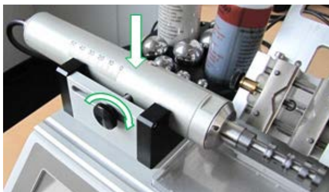
Fig. 22: Mounting motorized shaft on holder
