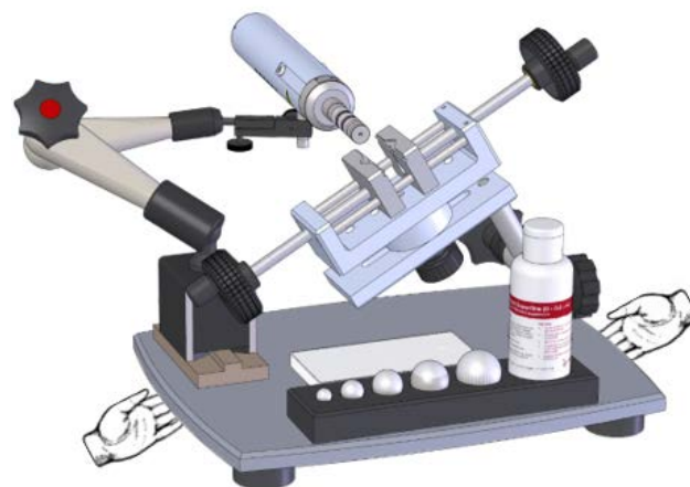
Fig. 90: Carrying the CAT 2i by the base plate
