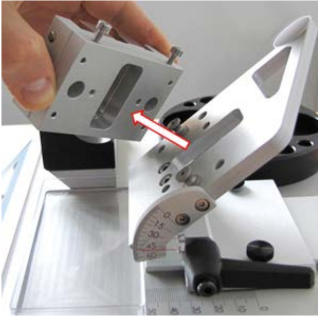
Fig. 73: Dismounting sample holder with support from table
