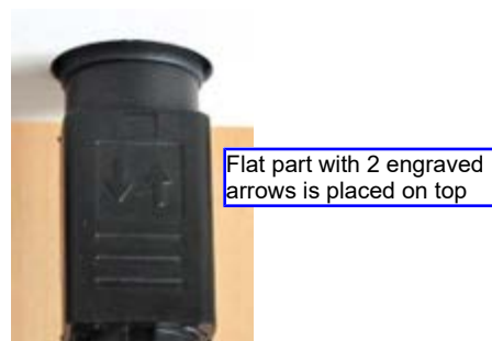
Fig. 15: Power supply MDJ-402 plug zoom
