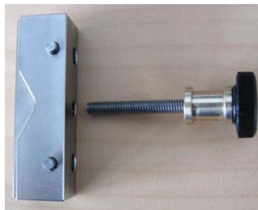
Fig. 77: Fully unscrewing hand screw from jaw
