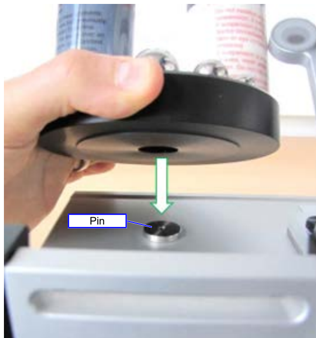
Fig. 23: Installing accessory holder on base plate
