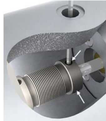
Fig. 86: Disconnection of the coupling from motor side
