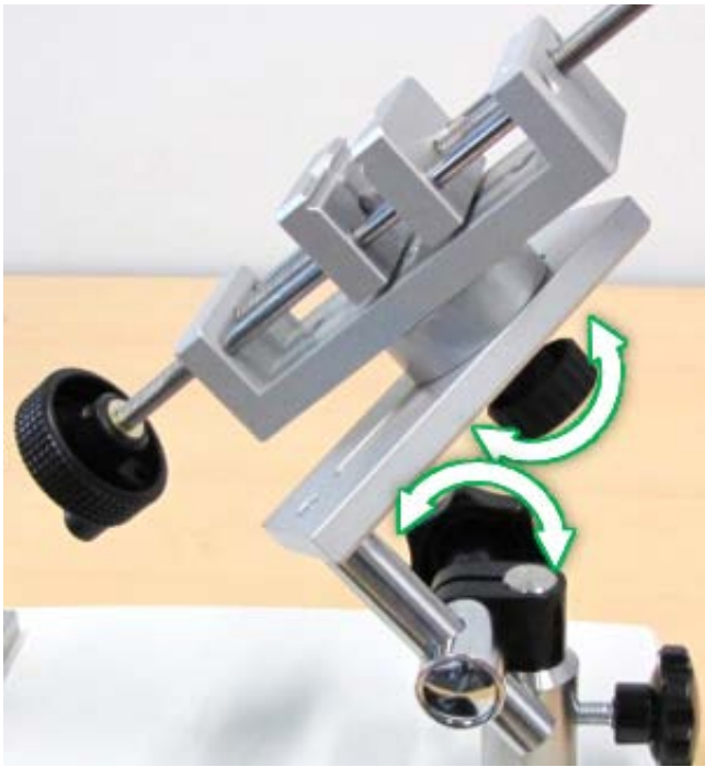
Fig. 68: Adjusting sample holder assembly
