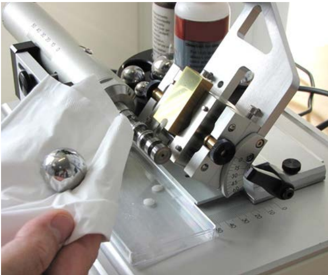
Fig. 64: Removing and cleaning the ball
