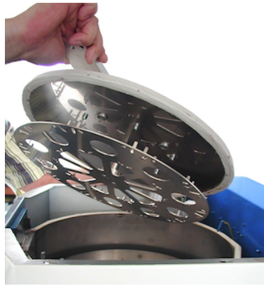
Fig. 38: Dismantling of the turntable assembly
