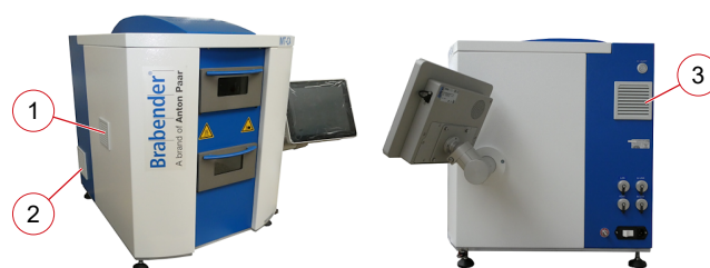
Fig. 39: Fans and ventilation grilles
