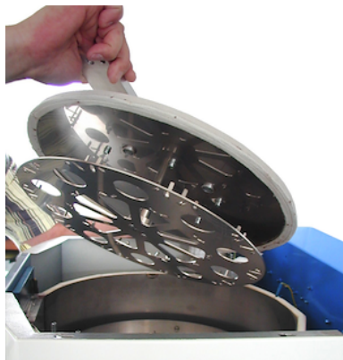
Fig. 24: Dismantling of the turntable assembly
