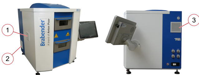
Fig. 25: Fans and ventilation grilles
