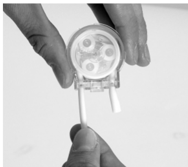
Fig. 13: Removing the hose
