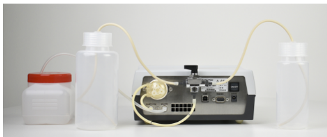
Fig. 7: Alex 501 – all hoses properly connected
