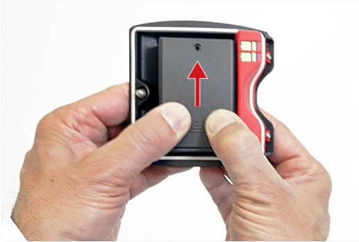
Fig. 10: Removing the cover of the battery compartment
