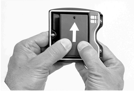
Fig. 11: Removing the cover of the battery compartment
