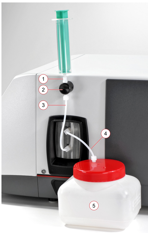
Fig. 2: All hoses mounted – syringe connected
