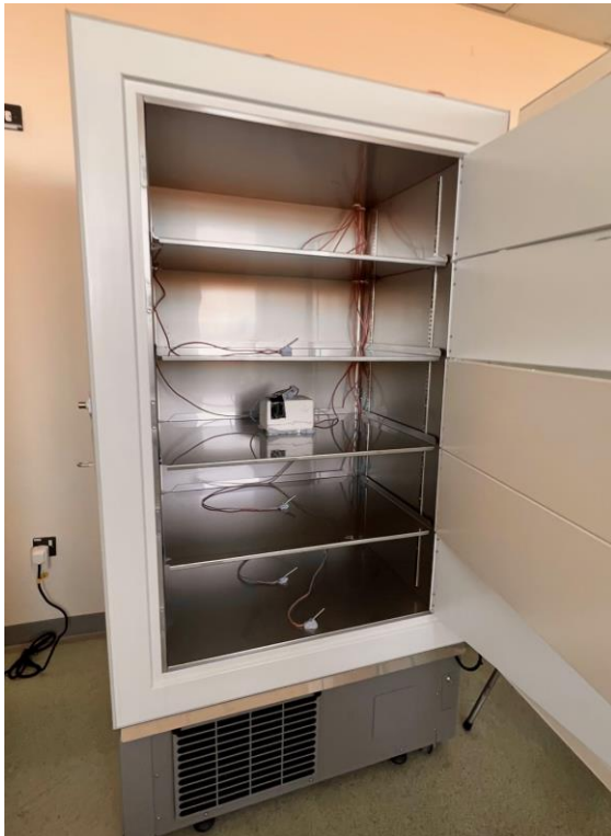
Figure 1. The F570h fitted with PT1000 probes and energy monitor.
