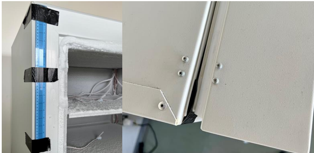
Figure 5. Left; securing the 45cm long ruler to the top left-hand side of the opened freezer created at 3.8mm gap (right) between the door seal and the freezer chamber. The obstructed seal spanned the entire height of the top freezer compartment (1) and ~50% of that of compartment 2.
