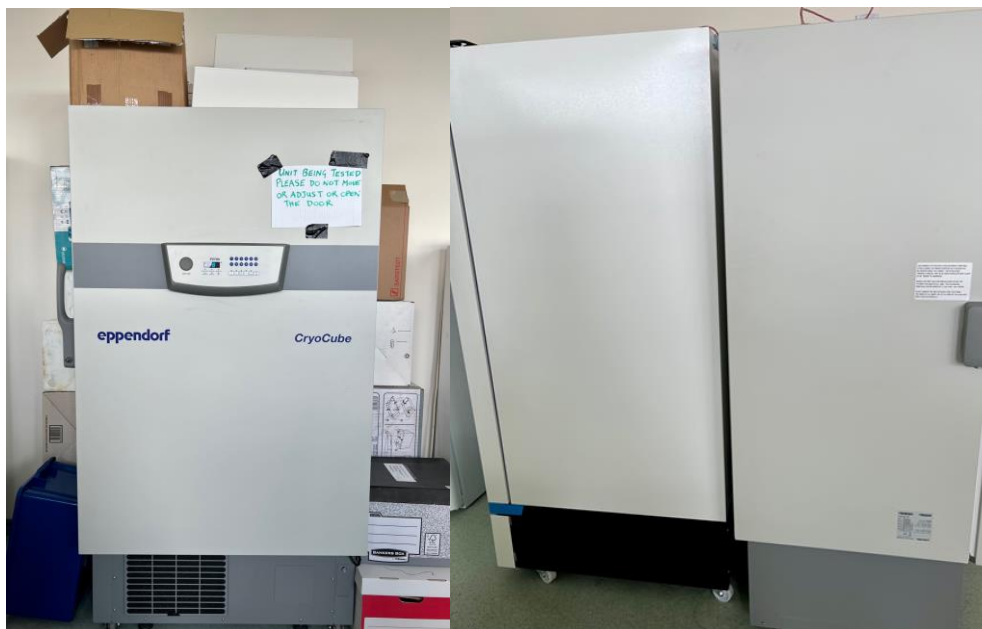
Figure 4. On the left, poor spacing. Placing a ULT freezer back to back with another is another form of poor spacing was examined separately.
